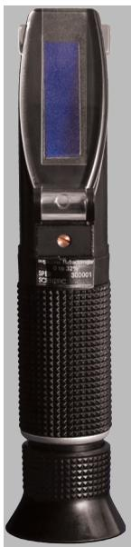
**Place a drop or two of a sample on the prism and read the results**
