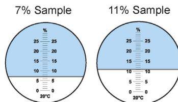
*Examples readings on Salt Refractometer 0 - 28% - 300006.*
