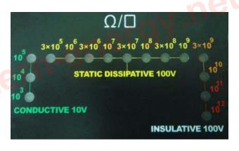
The test value is indicated on the LED display. Half decades provide greater accuracy by giving a closer approximation to the measurement value. An LED will brighten to the according test result. Colors signify the test value's function.
