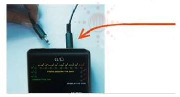
When the cables have been plugged into the appropriate sockets, the parallel probes under the meter disengage.
